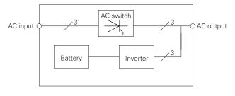
Fig. 4: Parallel processing system
