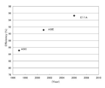
Fig. 1: Efficiency transition of the small capacity UPS
