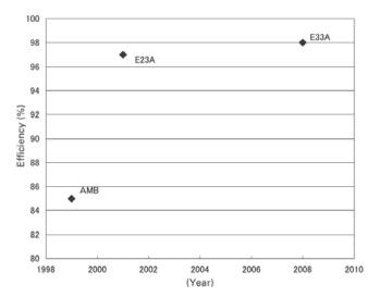
Fig. 3: Efficiency transition of the medium to large capacity UPS
