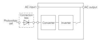
Fig. 6: Power conditioner circuit architecture
