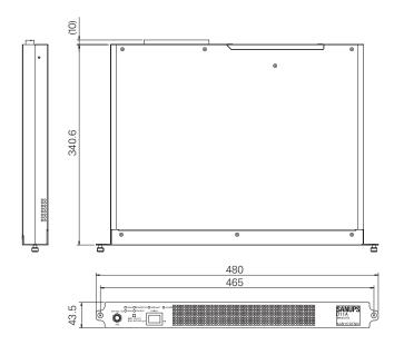
Fig. 10: External dimensions of the inverter unit
